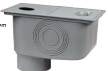
The drain cover is composed of the spout lid and full lid. The spout lid has pressed spots ready to prepare openings for spouts/pipes diameter Ø 50; Ø 80; Ø 90; Ø 100; Ø 110mm. Full lid enables inspecting and removal of dirt. The body of the under spout drain has a vertical outlet for sewage pipes diameter Ø 110mm. Inside there is a basket preventing the dirt from entering the sewage system and an anti-odour lid.
